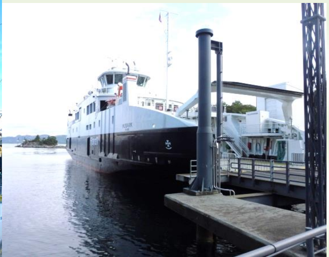
Battery operated ferry, charging port on the left photograph.
