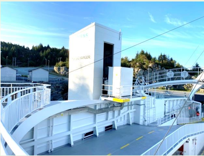
Battery operated ferry, charging port on the left photograph.
